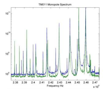
Figure 1: Monopole Spectrum, both couplers.
