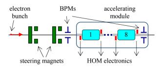
Figure 4: Steering Setup for HOM dipole experiment.
