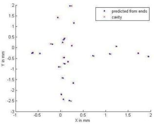
Figure 5: HOM beam position measurement from end cavities and middle cavity. RMS circular error is 24 microns.
