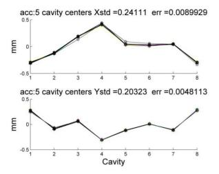
Figure 8: Alignment of TE111-6 cavity modes centers in module 5.
