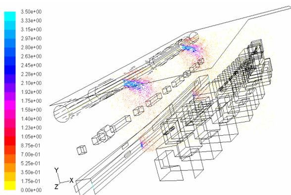
Figure 5: Simulated flow field in the storage ring tunnel of the TPS.
