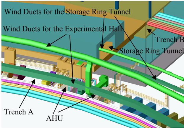
Figure 2: Layout of the storage ring tunnel and technical trenches of the TPS.
