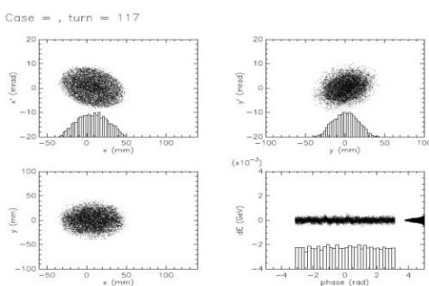
Figure 2: Beam distribution in phase spaces at injection end by a x-y anti-correlated phase space painting
