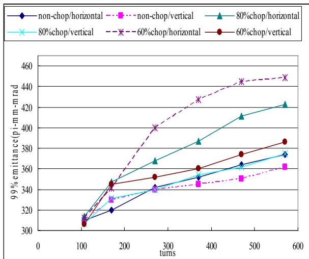
Figure 4 horizontal and vertical emittance growth
