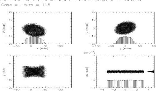
Figure 1: Beam distribution in phase spaces at injection end by a x-y correlated phase space painting
