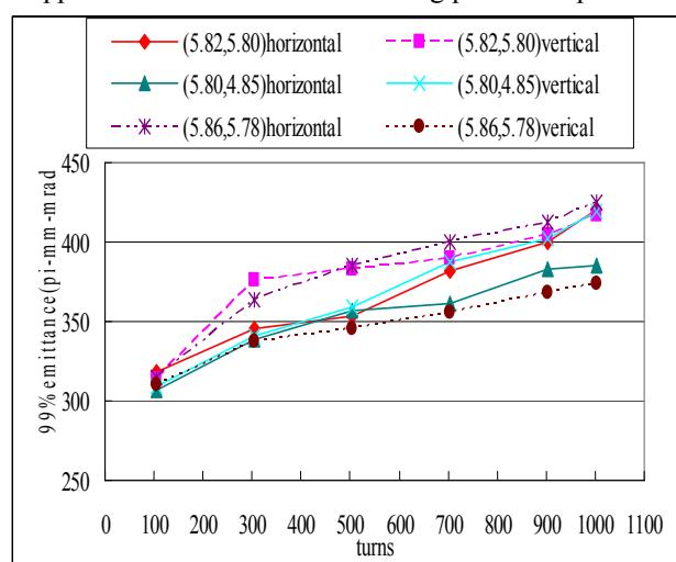
Figure 3 horizontal and vertical emittance growth for three of the working points
