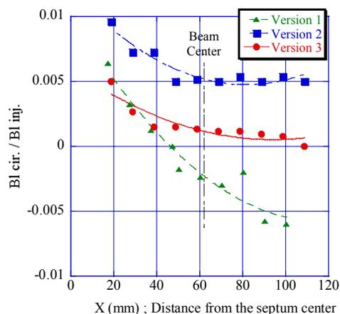
Figure 7: The measured value of transverse distribution of integrated magnetic field.
