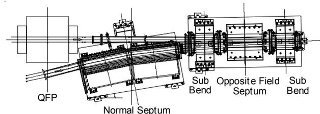
Figure 3: Outline of the injection system of JPARC main ring.
