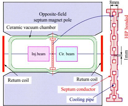
Figure 4: A transverse cross-sectional view of the injection system of JPARC main ring.
