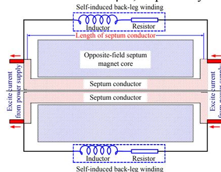
Figure 6: The self-induced back-leg windings to compensate error field induced by eddy current.
