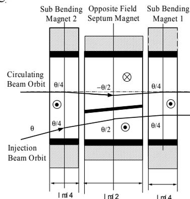
Figure 2: The concept of the opposite-field septum magnet system.
