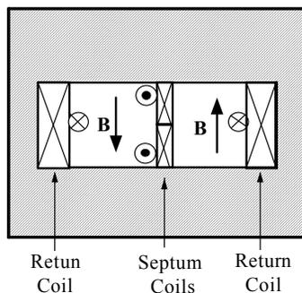
Figure 1: The fundamental concept of the opposite-field septum magnet.
