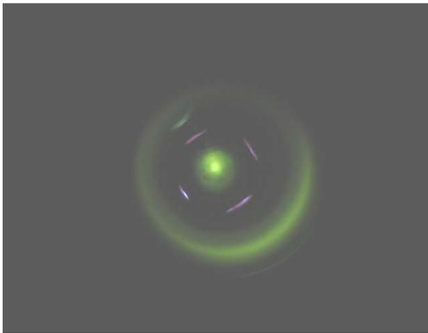
Figure 3: Image of electron beam imprint on phosphor scintillator (3 pulse integration), electron beam diameter (represented by central bright spot) was 3 mm
