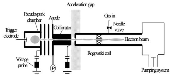
Figure 7: Schematic diagram for the post-acceleration experiment of the pseudospark electron beam
