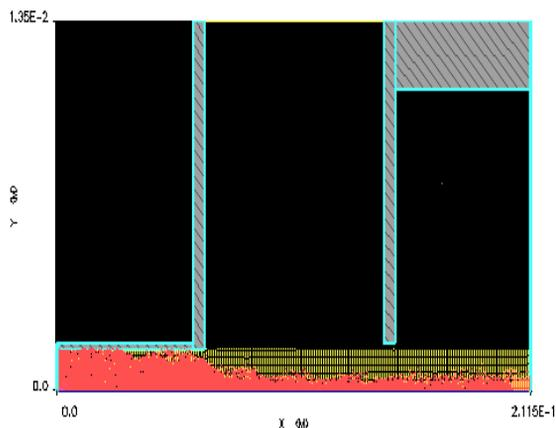
Figure 9: Beam propagation with a plasma of density  $6 \times 10^{12} \text{cm}^{-3}$  filling the channel beam 200A, 200V, red electrons, yellow- plasma.
