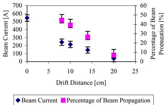
Figure 4: Electron beam current and its propagation percentage along the axis after the anode
