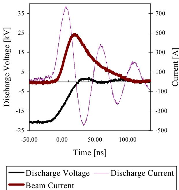
Figure 2: A temporal evolution of the beam produced from a three-gap pseudospark discharge chamber
