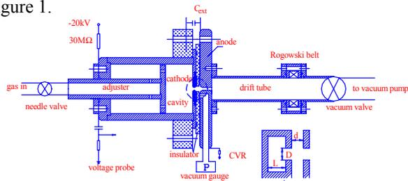
Figure 1: Pseudospark discharge and beam extraction experiments
