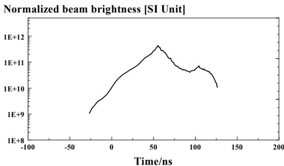
Figure 5: Measured beam brightness from a 3-gap pseudospark discharge
