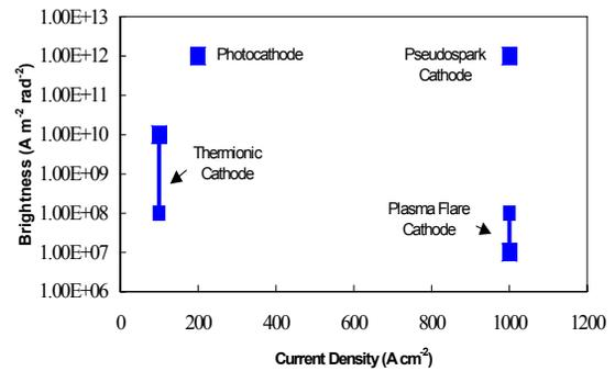
Figure 6: Brightness as a function of current density for various electron beam sources
