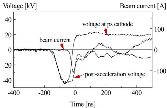
Figure 8: Typical record of the time-correlated pseudospark discharge voltage, beam current and the acceleration voltage pulse
