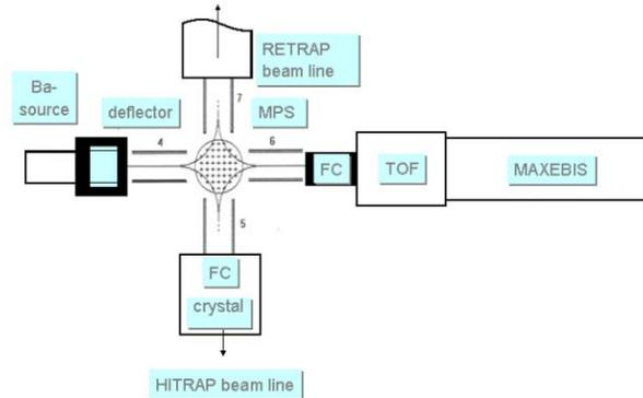
Figure 3: Front-end setup of the MAXEBIS beam line. FC= faraday cup.
