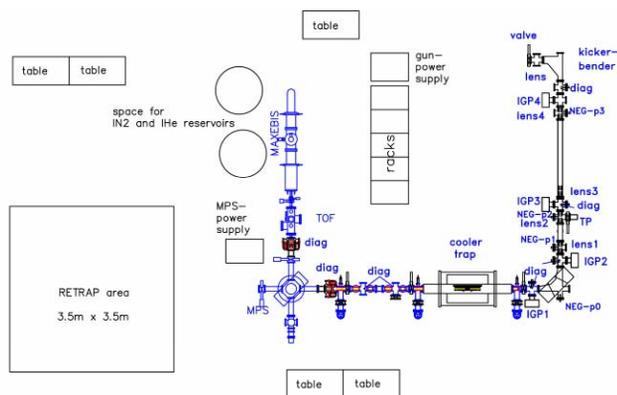
Figure 1: Setup of the test injector beam line for the HITRAP cooler trap vertical beam line and RETRAP and for charge breeding experiments, built up outside GSI at the Heckhalle.
