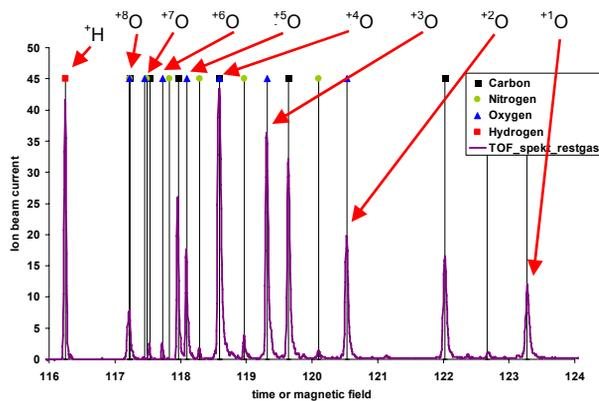
Figure 5: Residual gas TOF spectrum of the MAXEBIS
