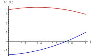
Figure 6: Magnet fields  $B_d$  (red) and  $B_f$  (blue) versus momentum  $p$
