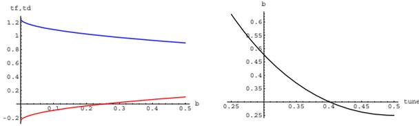
Figure 3: Bend angle ratios  $\theta_{f1}/\theta$  (red) and  $\theta_{d1}/\theta$  (blue) versus  $b$ .
