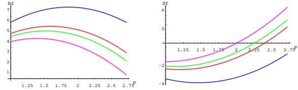
Figure 3: Field integral versus momentum in D element (left) and in F element (right). Colour coding as above.
