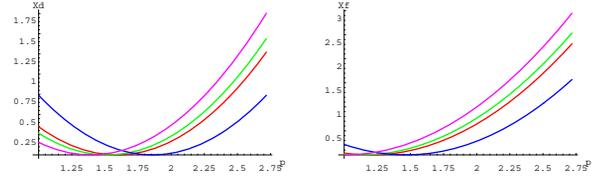
Figure 2: Radial closed orbit versus momentum in D element (left) and in F element (right). Colour coding: optimize  $\Delta x_d$  (blue),  $\mathcal{B}_f$  (green),  $\Delta\mathcal{L}$  (red),  $\mathcal{B}_m$  (magenta).
