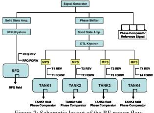
Figure 7: Schematic layout of the RF power flow
