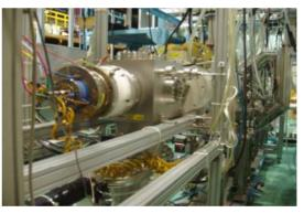
Figure 2: PEFP Proton Injector
