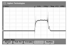
Figure 3: Beam signal at the LEBT exit (1mA/div. 200us pulse)
