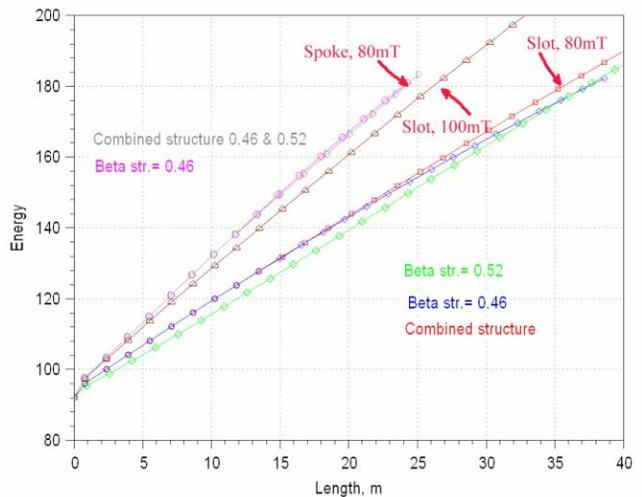
Figure 5: Energy gain in slot and spoke structures.
