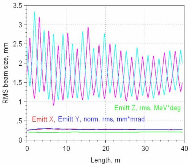
Figure 3: Beam envelopes and emittances behaviour.
