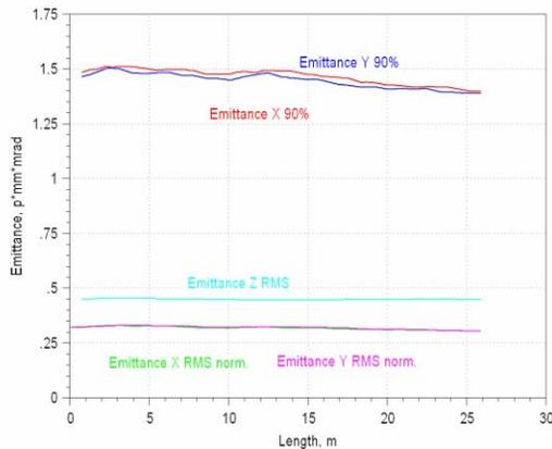
Figure 7: Emittances behaviour in spoke structure.
