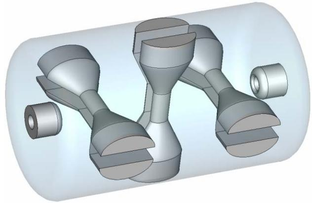
Figure 4: Slot structure type with improved electro-dynamical parameters.
