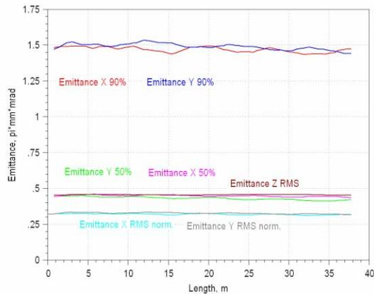
Figure 6: Emittances behaviour in slot structure.
