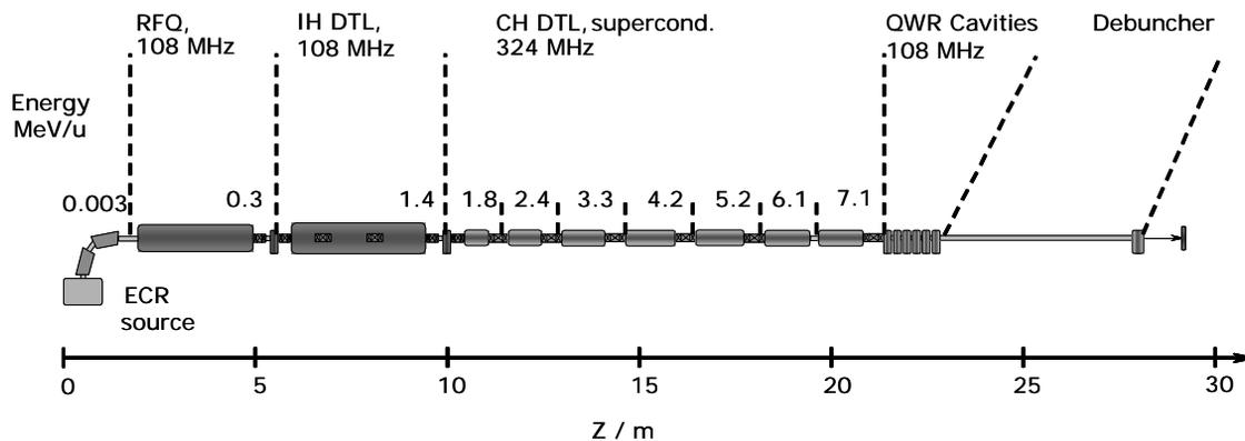
Fig. 7: Proposed layout of a cw-superconducting LINAC. [4]
