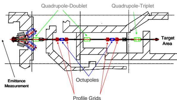
Fig. 4: Upgrade of the beam transport line to the SHIP; two quadrupole duplets provide for a sufficient beam spot (measurable at four SEM-profile grids) performing rectangular profile shaping with two octupole lenses.
