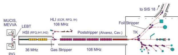
Fig. 2: Schematic overview of the GSI UNILAC and experimental area.
