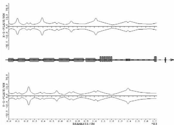
Fig. 8: First beam dynamics layout (transversal beam envelopes) of the sc-CH-drift tube linac.
