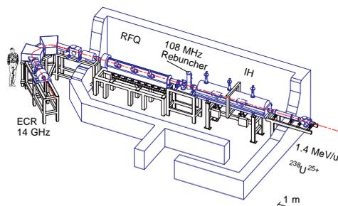
Fig. 3: Status Quo of the High Charge State Injector.
