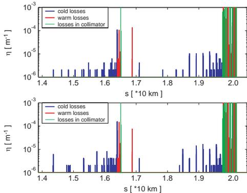
Figure 2: Beam 2 loss patterns for injection optics from the end of arc 5-6 to the end of IR7 for an ideal machine (top) and a ± 4 mm horizontal orbit perturbation (bottom). The quench level is  $10^{-3}$  protons.m<sup>-1</sup>. Beam 2 goes from right to left.
