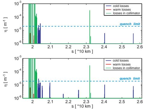
Figure 3: Beam 1 loss patterns for collision optics from the start of IR7 to the end of arc 8-1 for an ideal machine (top) and a horizontal orbit perturbation of ± 4 mm in the arcs and ± 3 mm in the insertion regions (bottom). Beam 1 goes from left to right.
