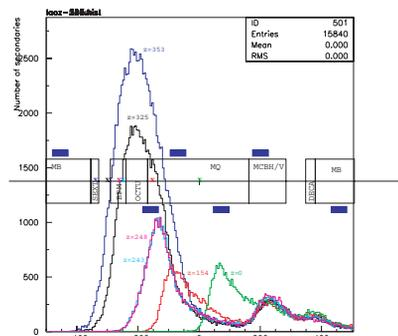
Figure 5: Shower development in the cryostat of a quadrupole. The positioning of the detectors (blue boxes) has been optimized to catch losses (colored curves) and to minimize uncertainty of ratio of energy deposition in coil and detector (courtesy of L. Ponce).
