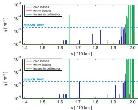
Figure 4: Beam 2 loss patterns for collision optics from the end of arc 5-6 to the end of IR7 for an ideal machine (top) and a horizontal orbit perturbation of ± 4 mm in the arcs and ± 3 mm in the insertion regions (bottom). Beam 2 goes from right to left.
