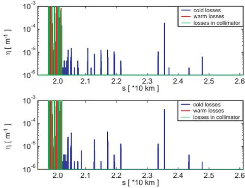
Figure 1: Beam 1 loss patterns for injection optics from the start of IR7 to the end of arc 8-1 for an ideal machine (top) and a ± 4 mm horizontal orbit perturbation (bottom). The quench level is  $10^{-3}$  protons.m<sup>-1</sup>. Beam 1 goes from left to right.
