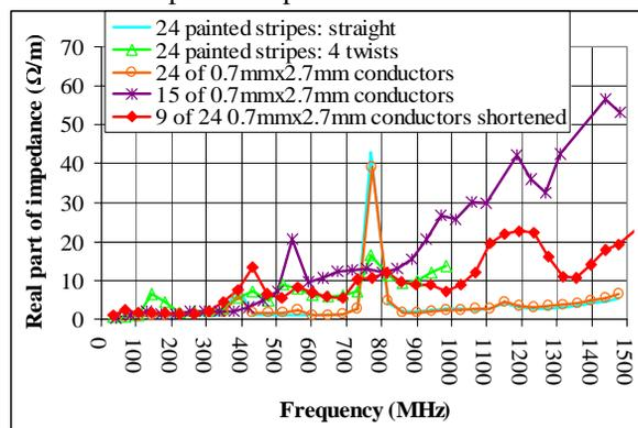
Figure 4: Real part of measured complex impedance, of an LHC injection kicker, for various beam screens.
