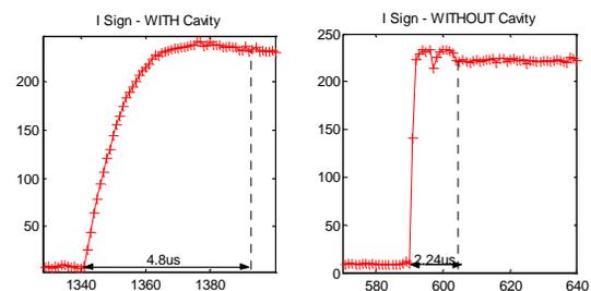
Figure 7. PI Loop Step response with &amp; without cavity
