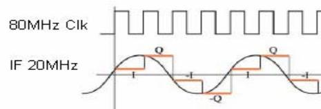
Figure 5: Digital IQ Demodulation
