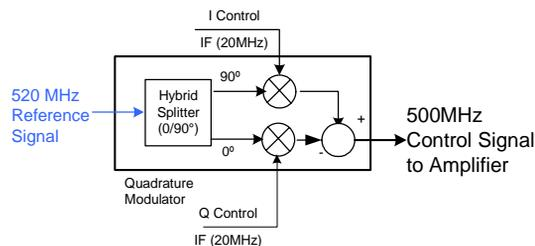
Figure 6. Upconversion of control signals to 500MHz
