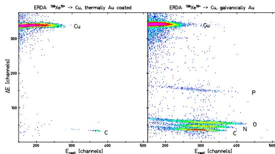
Figure 4: ERDA spectra of the two gold coated copper samples.
