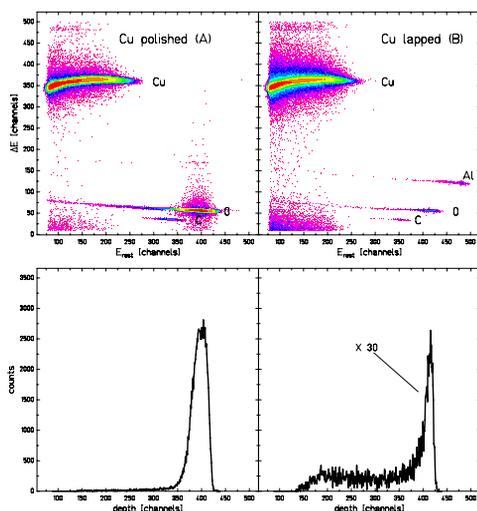
Figure 3: ERDA spectra of the copper samples. Left: polished with a huge oxide layer, right: lapped with few contaminations.
