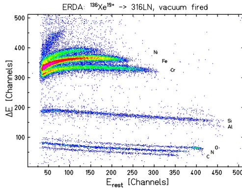
Figure 1: ERDA raw spectrum of the 316LN sample. Each  $\Delta E$  branch represents an element while  $E_{rest}$  is a function of the depth in the target.
