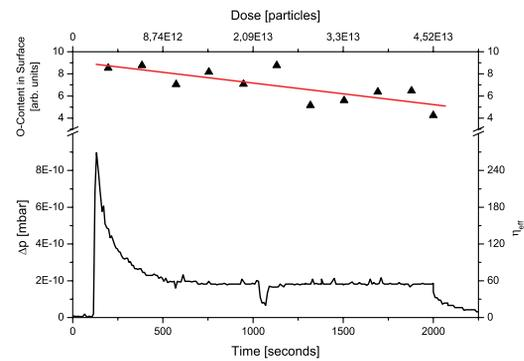
Figure 2: Dose dependent evolution of the oxide layer (top) and the desorption yield (bottom).
