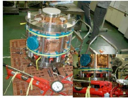
Figure 2: Setup for the TIG welding with pressurization. Eight hydraulic cylinders are put on the lower endcap.
