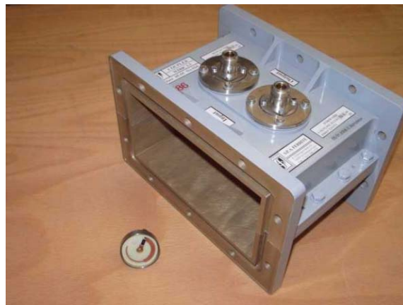
Figure 5: The directional coupler and stripline head.
