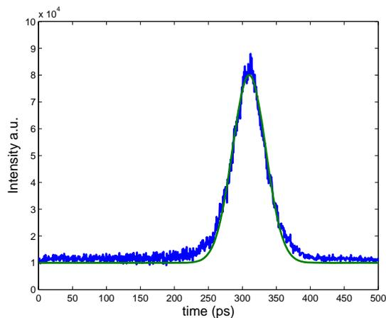
Figure 4: Profile of the stored beam, and Gaussian fit. The bunch length is measured at  $\sigma_{r.m.s} \approx 24$  ps.
