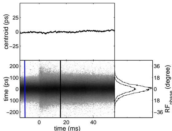
Figure 2: Matched energy and phase at injection, and stored beam. The bunch length is  $85 \text{ ps}$  shortly after injection, and  $70 \text{ ps}$  just before injection (that is after  $200 \text{ ms}$ ), which shows that the beam is still oscillating then.
