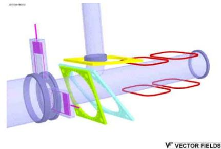
Figure 4: CSR electron beam diagnostics. The ion beam circulates from the right to the left. The electron beam comes through the vertical tube and is bent to the left. The solenoid with the x and y-wire scanners at its entrance is located to the left. The magnetic shielding around the cooler is not seen in the picture.
