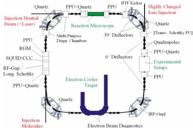
Figure 1: Layout of the CSR beam diagnostics system.
