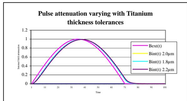
Figure 2: Effect of ±10% variation of coating thickness.
