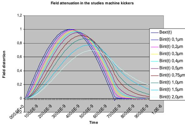
Figure 3: Pulse signal attenuation of the machine study kicker versus the coating thickness.
