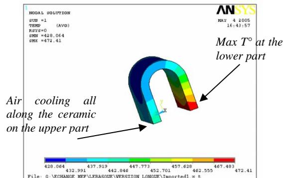
Figure 5: Thermal calculation of the ceramic vacuum chamber for 500mA and  $0.2\mu\text{m}$ .
