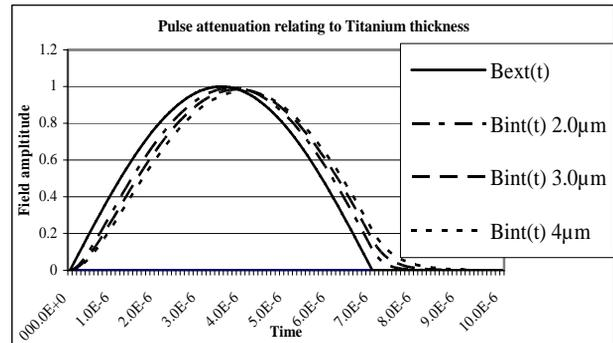
Figure 1: Pulse signal attenuation of the injection kicker versus the coating thickness.
