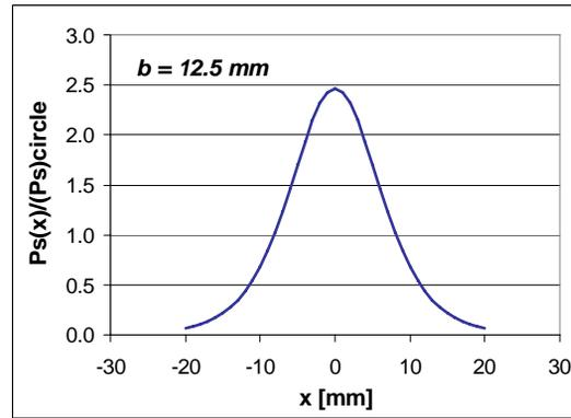
Figure 4: Transverse distribution of the ratio between the power density on a 2 plates model chamber and its density on a circular chamber.
