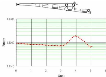
Figure 7: Pressure profile for the B1-chamber. Three 400 L/s pumps are represented by the three circles in the drawing of the triangular shape B1-chamber.
