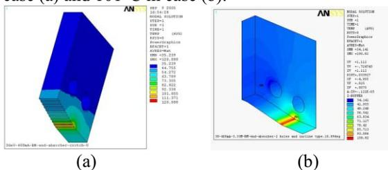
Figure 5: Simulation of the thermal distribution on the downstream Al absorber with interior cooling in cases of irradiation surfaces with (a) saw-tooth structure, and with (b) incline surface.
