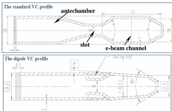
Figure 2: Cross sections of the standard profile and for the dipole chamber profile, respectively.
