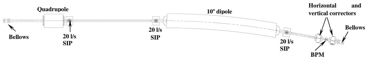
Figure 5: the vacuum layout of the unit cell of the booster synchrotron
