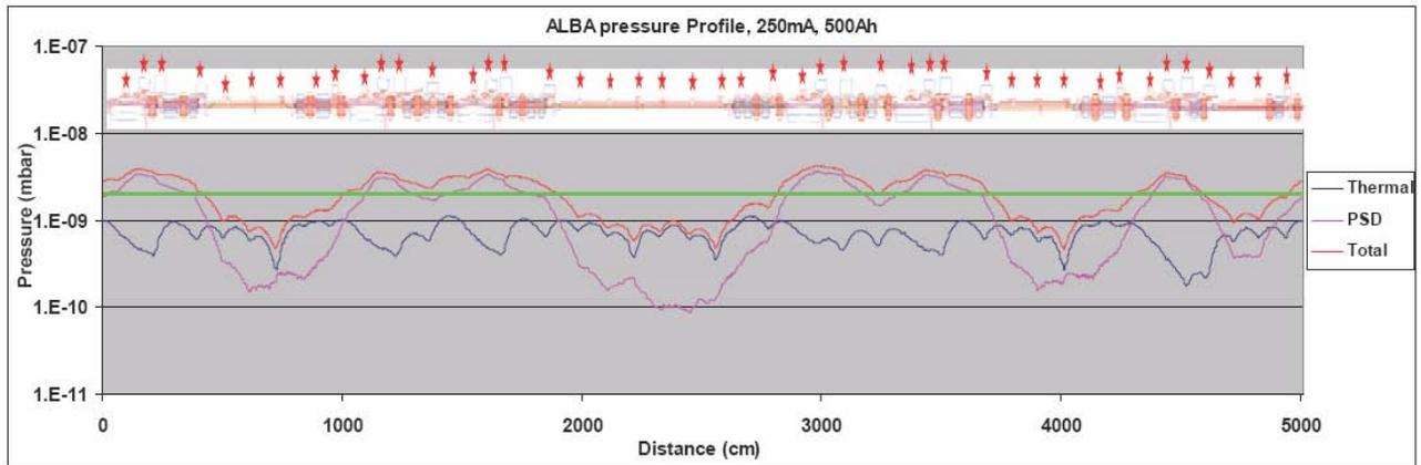
Figure 4: The pressure profile of ALBA storage ring at nominal current 250 mA after 500 Ah.
