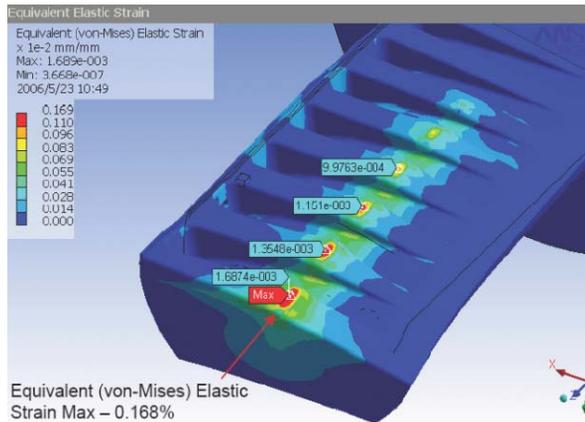
Figure 3: the equivalent von-Mises strain for the critical absorber (Glidcop®).
