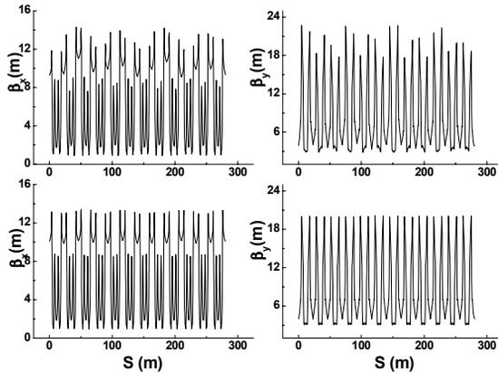
Figure 3: Predicted beta functions before (top plot) and after correction (bottom plot). It is seen that after correction beta functions became very close to the designed values and near twelve-fold symmetry of the ring was restored.
