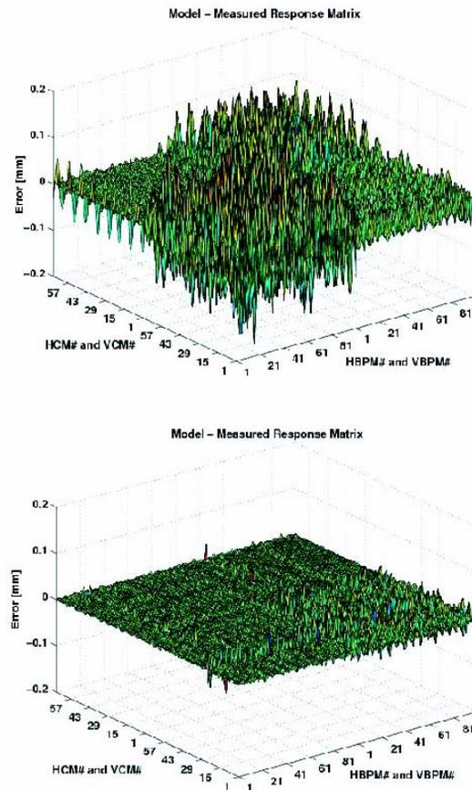
Figure 1: (a) Difference between the measured response matrix and the model response matrix before correction (upper plot). (b) Difference between the measured response matrix and the model response matrix after correction (lower plot).
