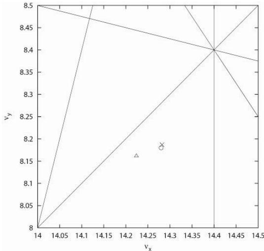
Figure 4: Measured tune values and resonance diagram. Allowed resonances up to the 5<sup>th</sup> order are shown as solid lines. A circle mark indicates the design tunes (14.28, 8.18), the triangle mark shows the tunes before correction and the cross mark indicates the tunes after correction.
