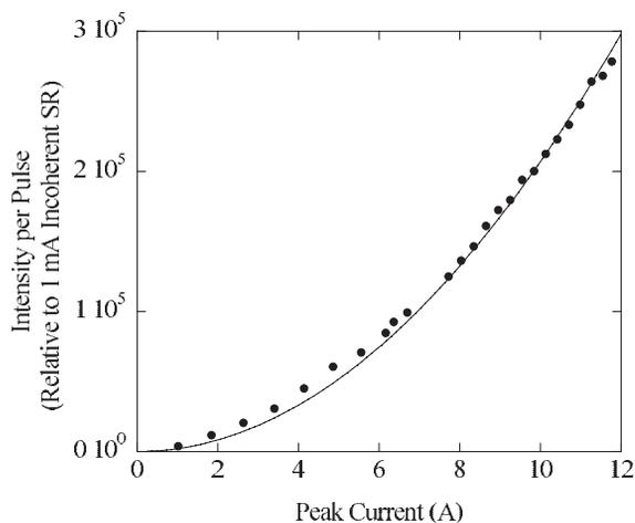
Figure 5: Terahertz intensity per pulse versus peak current of electron bunch. The solid line is a best-fit square curve.
