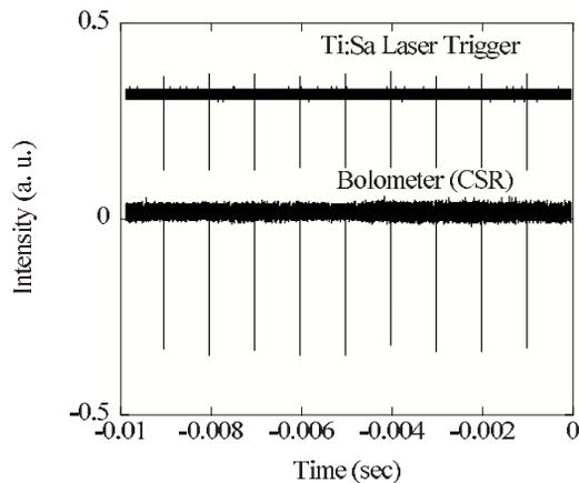
Figure 3: Terahertz pulses induced by the laser injection. The lower curve is the output signal (negative) of the terahertz detector and the upper the laser trigger signal.
