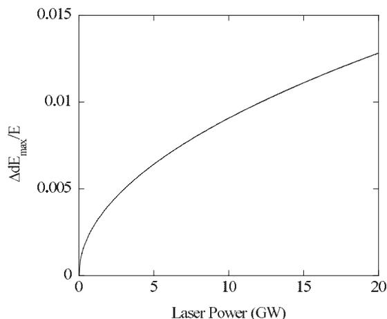
Figure 2: Amplitude of energy modulation versus laser peak power estimated by assuming appropriate focussing of the laser beam in the modulator.
