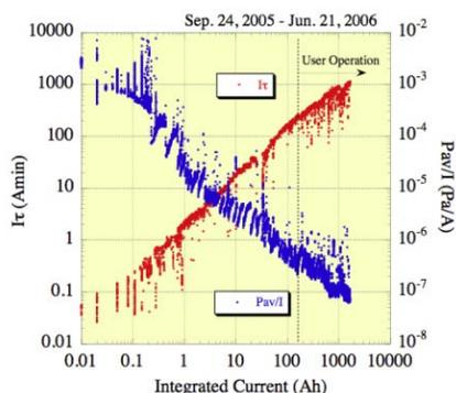
Figure 8: Observed data of the average pressure and the beam lifetime from the start of the recommissioning.
