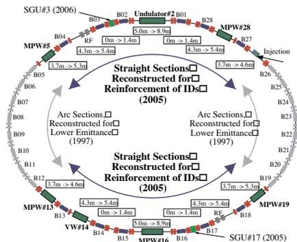
Figure 1: Reconstructed regions in the PF ring straight sections upgrade project.
