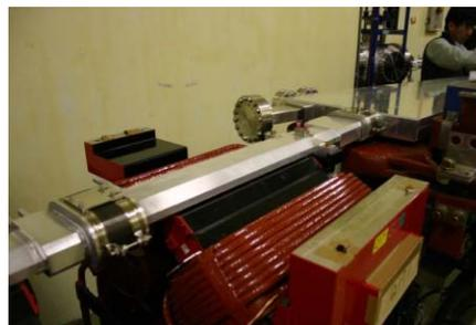
Figure 4: Photograph of one of the new ducts.
