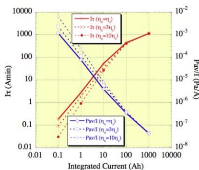
Figure 7: Results of the estimations of the average pressures and the beam lifetimes after the reconstruction.
