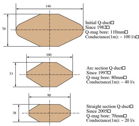
Figure 3: Transition of the Q-duct cross-sections.
