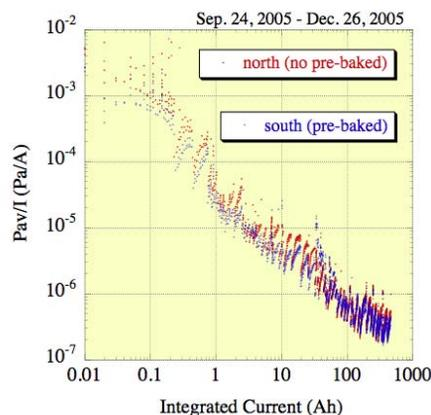
Figure 9: Observed average pressures in the northern (no pre-baked) and in the southern (pre-baked) straight sections.
