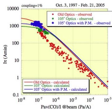
Figure 6: Observed and calculated lifetimes as a function of the CO-equivalent average pressure along the beam.
