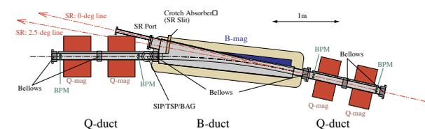
Figure 2: Typical composition of the new vacuum ducts.
