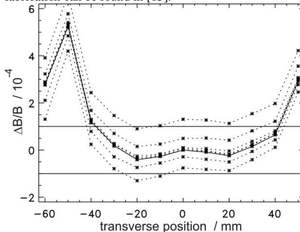
Figure 3: Measured homogeneity of the magnetic field in the central region of the MLS bending magnets according to ref. [16]. The solid line is at the longitudinal center of the magnet, the dotted lines have an offset of 5 mm, 10 mm and 15 mm upstream and downstream, respectively.
