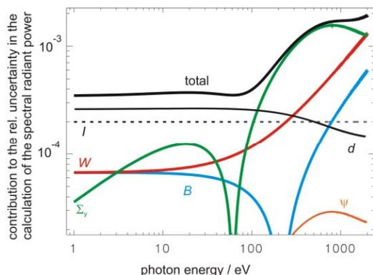
Figure 4: Relative uncertainty in the calculation of the spectral photon flux of the MLS. The uncertainty of the input parameters is according to Tab. 1.
