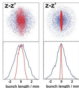
Figure 5: Plot of longitudinal beam phase space ( $z, z'$ ) at two different dipole beam ports of two bunches of different length (red, blue). The lower part shows, that the projected rms bunch length of 1 mm is achieved at both places (blue), 10 times shorter bunches (red) only at beam port #9 (see Fig. 2).
