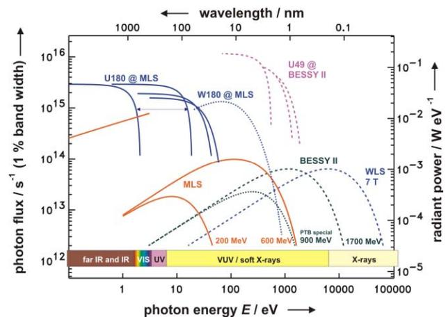
Figure 1: Spectrum of the MLS as compared to BESSY II. With the electron storage rings MLS and BESSY II (including a 7 T WLS), PTB can use synchrotron radiation in the spectral range from the FIR up to the hard X-rays for photon metrology.
