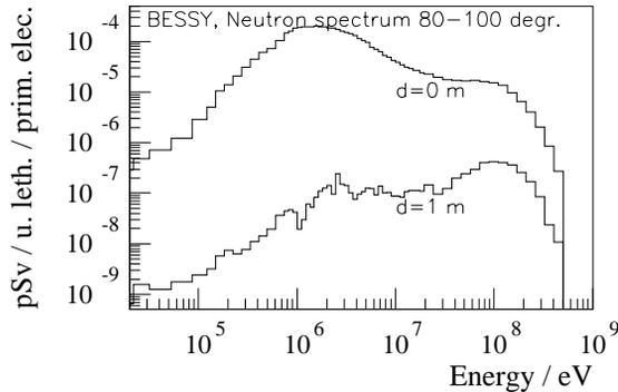
Figure 3: Neutron spectra at  $90^0$ , Al-Target
