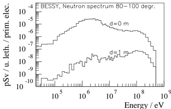
Figure 4: Neutron spectra at  $90^0$ , thin Fe target
