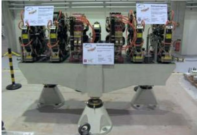
Figure 4: First assembled achromat girder in May
