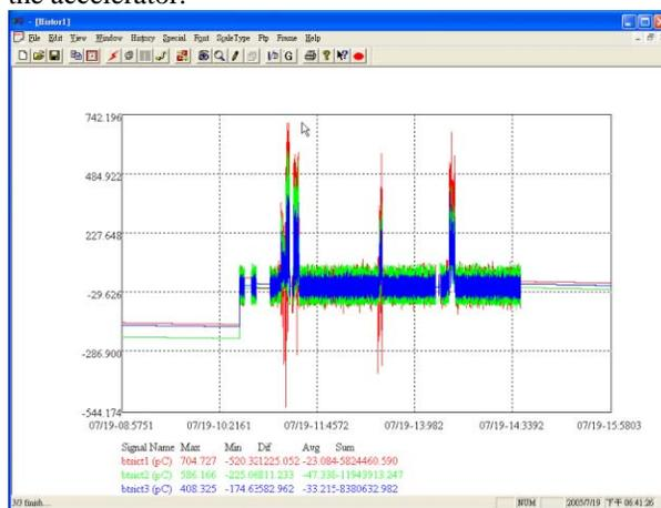
Figure 8: Signal after EMI reduction.
