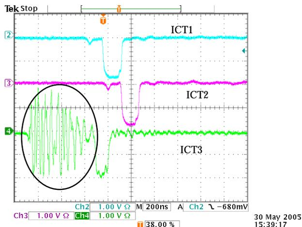
Figure 3: The signals measured by ICTs.
