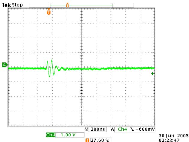
Figure 7: Noise picked up after add the spray ground routes.
