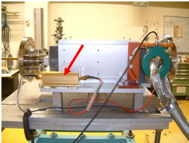
Figure 4: The real testing set-up of the secondary coil upon the main coil. The resistor is pointed.
