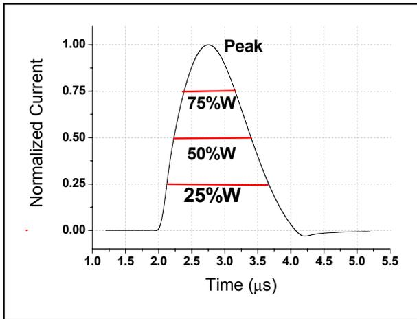
Figure 2: The proposed check points and pulse widths characterizing the shape of each pulse.
