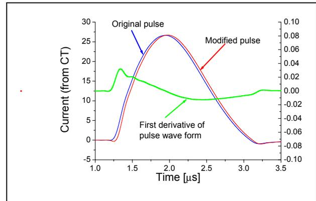
Figure 5: A typical pulse shape of the current and its modification
