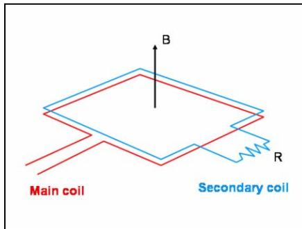
Figure 3: The secondary coil (cyan) with a resistor shunted to modify the magnetic field caused by the main coil (red).
