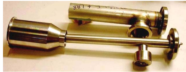
Figure 4: Welding tooling used to minimise deformation.
