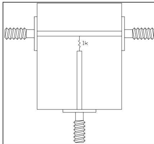
Figure 9: Schematic of high impedance pickoff.
