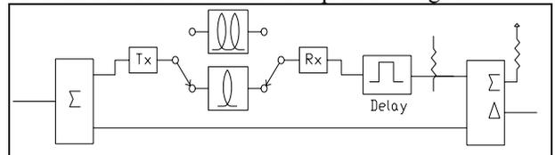
Figure 6: Schematic of the comb filter.
