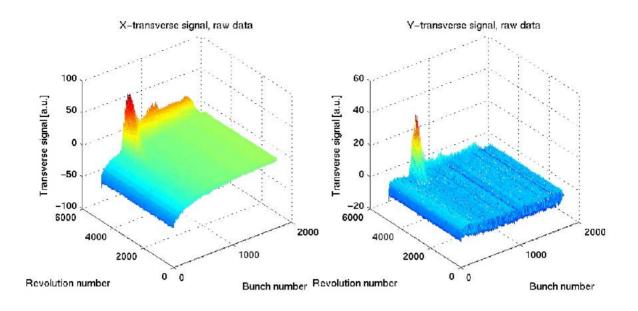
Figure 4: 3d plot of the transverse beam position.
