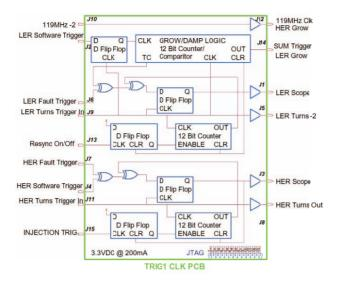
Figure 3: Trigger logic implemented in the CPLD.
