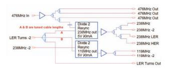
Figure 2: Timing logic for the GaGe-82G cards.
