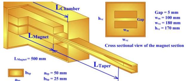
Figure 4: 3D-Model of the in-vacuum permanent magnet undulator.
