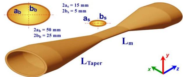
Figure 1: Tapered elliptical vacuum chamber for superconducting small-gap undulator.
