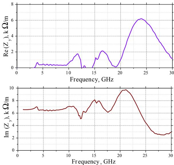
Figure 3: Real and imaginary parts of the transverse impedance in the tapered elliptic vacuum chamber ( $L_{Taper}=180\text{mm}$ ). Impedances correspond to FFT of the computed wakepotential up to  $s=1.5\text{m}$ .
