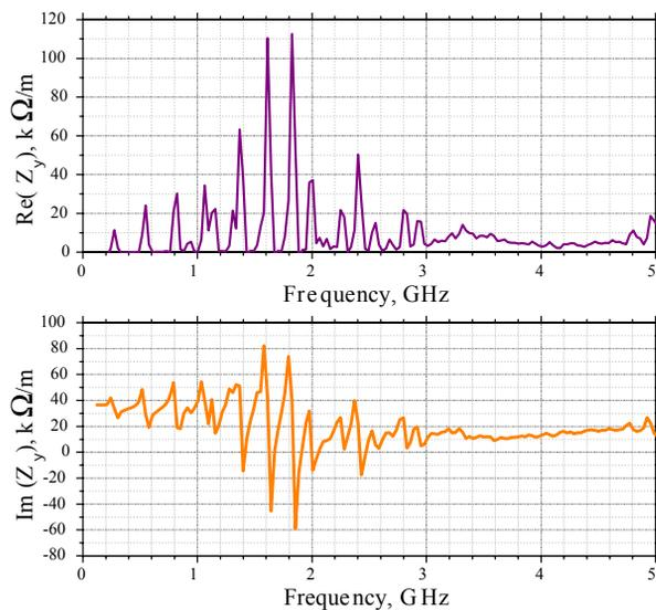
Figure 6: Low frequency behavior of the real and imaginary parts of the transverse impedance in in-vacuum permanent magnet undulator. Impedances correspond to FFT of the computed wakepotential up to  $s=7\text{m}$ .
