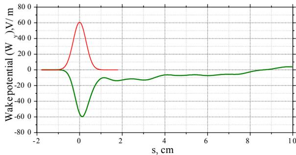
Figure 5: Short-range transverse wakepotential in in-vacuum permanent magnet undulator.
