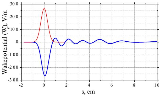
Figure 2: Transverse wakepotential in the tapered elliptic vacuum chamber ( $L_{Taper}=180\text{mm}$ ).
