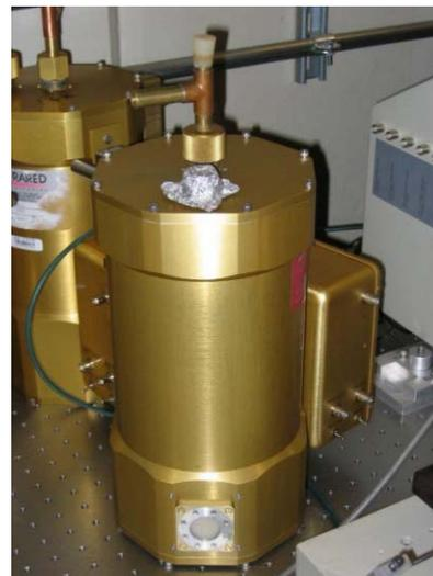
Figure 1: Infrared Laboratories 4.2 K Si bolometer.
