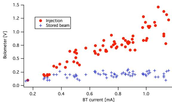
Figure 6: Bolometer signal from injection a stored beam as a function of the bunch current (injection transfer line current monitor).
