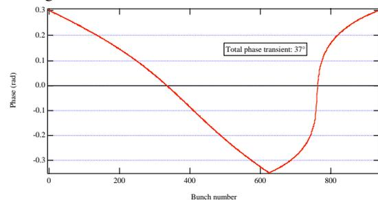
Figure 2: Synchronous phase along the bunch train (33% gap).
