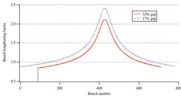
Figure 3: Bunch lengthening factor for the nominal gap (33%) and a halved gap (17%).
