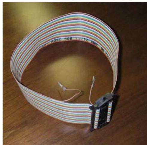
Figure 1: A solenoid made of a flat cable.
