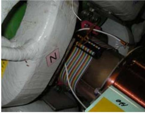
Figure 2: A solenoid installed in a quadrupole magnet.
