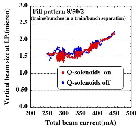
Figure 5: Vertical beam size at I.P. as a function of a total beam current with or without Q-solenoids.
