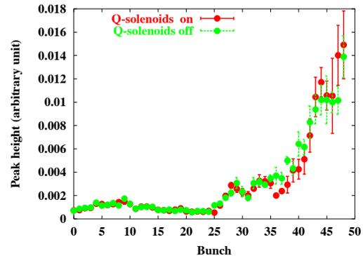
Figure 4: Peak height of vertical sidebands along the train with or without Q-solenoids.
