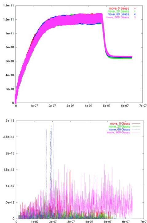
Figure 6: Simulated electron cloud density as a function of time in sec at four different solenoid strengths (0, 20, 60 and 600 G) by ECLLOUD. Top: the electron line density in units of  $m^{-1}$ , bottom: the central electron density in units of  $m^{-3}$ . Bunch separation is 2 rf buckets. The strength of a quadrupole is 5 T/m.
