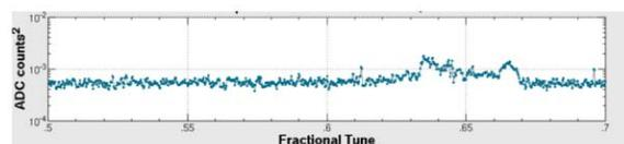
Figure 3: Power spectrum of the vertical dipole oscillation with or without Q-solenoids.
