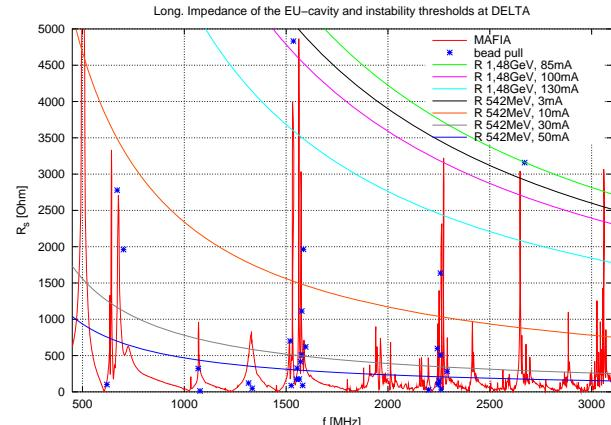
Figure 1: Computed and measured longitudinal impedances of the HOM-damped EU-cavity [1] together with threshold impedances of DELTA at several currents and energies.
