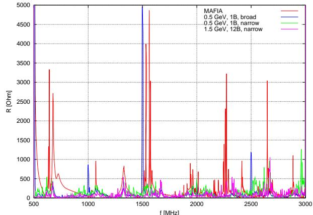
Figure 5: Impedance spectra of the EU-cavity at single-bunch operations from narrow- and broadband measurements and 12-bunch narrowband compared to MAFIA results.
