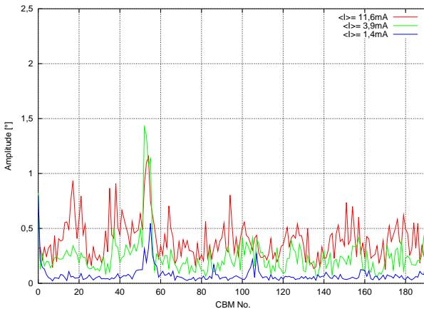
Figure 2: CBM spectra at 542 MeV and mean beam currents of 11.6 mA (red) 3.9 mA (green) 1.4 mA (blue), taken with the EU-cavity installed.
