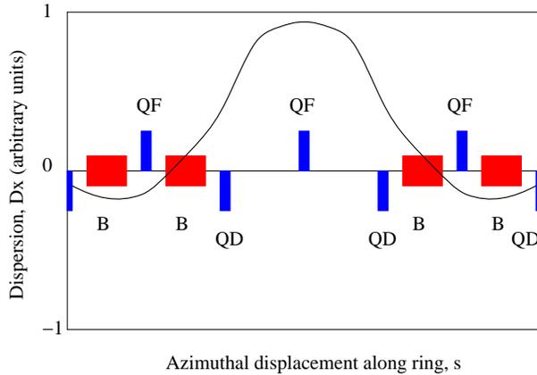
Figure 1: 3-cells missing-dipole low-momentum-compaction lattice module. B, QF, and QD denote dipole, focusing, and defocusing quadrupole magnets, respectively. The horizontal phase advance across the module is approximately  $270^\circ$ .
