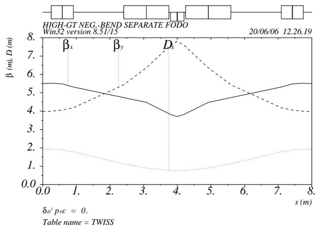
Figure 6: High- $\gamma_T$  negative-bend lattice with  $95.4^\circ$  horizontal phase advance.
