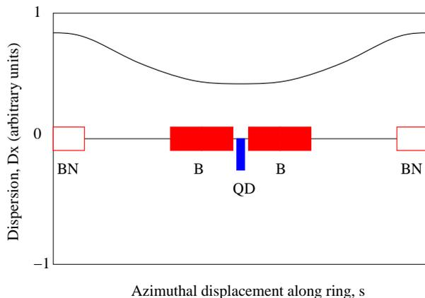
Figure 2: Negative-bend low-momentum-compaction lattice. B, BN, and QD denote dipole, negative-bend dipole, and defocusing quadrupole magnets, respectively. The horizontal phase advance across the module is usually below  $127^\circ$ .
