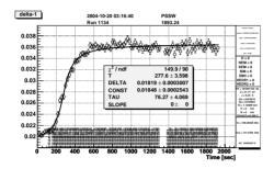
Figure 3: Long-drawn jump at the reduced strength of depolarizer. Duration time of the jump corresponds to  $\sim 3.5$  keV interval in the energy scale and is determined by the spin frequency linewidth.
