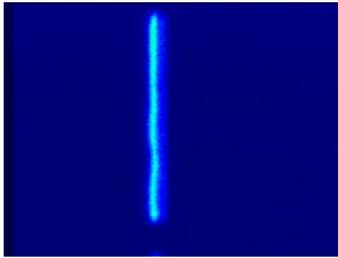
Figure 2: A pico-second streak camera image. Horizontal axis represents the beam motion in the vertical direction. The full extent of vertical axis is  $1\mu s$ .
