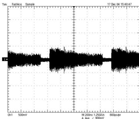
Figure 3: Bunch train signal after the ion instability was generated. The horizontal time division is 200ns. The ring revolution time is  $0.936\mu s$ . The unfilled part is ion-clearing gap.
