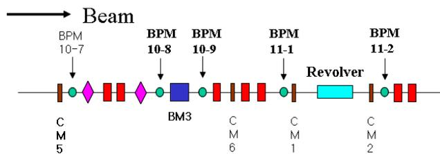
Figure 6: Lattice around the revolver and the upstream dipole magnet. CM represents the corrector magnet and the red color box the quad.
