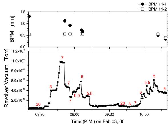
Figure 7: Upper figure: vertical beam position change around the revolver; lower figure: the resultant change of the revolver vacuum. The red-colored numbers in the lower figure denote the gap size.
