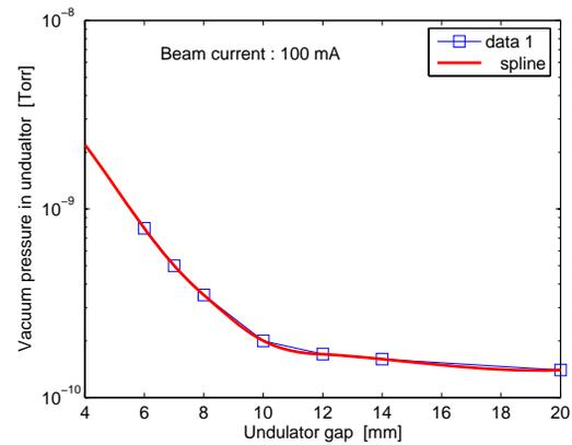
Figure 4: The vacuum pressure in the revolver as a function of the revolver gap.
