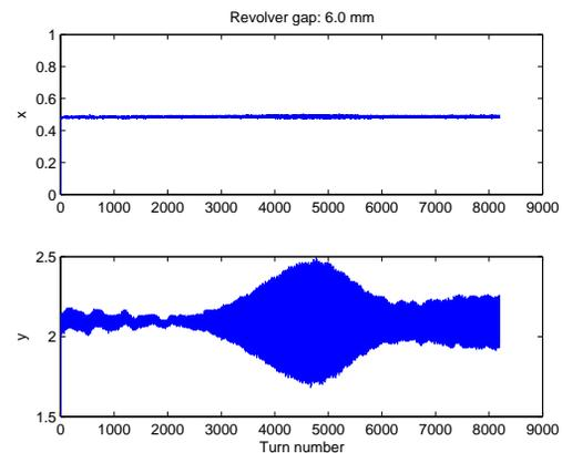
Figure 5: The horizontal (x) and vertical (y) beam oscillation obtained by a turn-by-turn digital BPM when the gap was set at 6 mm. The unit of vertical axis is mm and one turn in horizontal axis corresponds to  $0.936\mu s$ .
