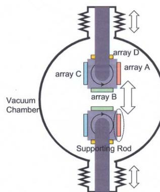
Figure 1: Permanent magnet array structure of the in-vacuum revolver (RIVXUN).
