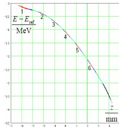
Figure 3: Longitudinal momentum distribution in front of the first bunch compressor. Different slices of the bunch are colour coded for easier identification of what happens during stage of compression.
