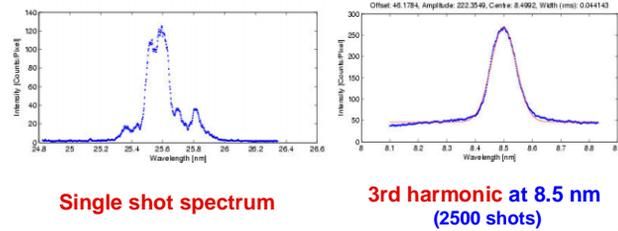
Figure 11. Single shot spectrum at 25 nm wavelength (1<sup>st</sup> harmonics) (left), and corresponding 3<sup>rd</sup> harmonics spectrum (right).
