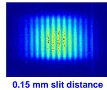
Figure 12. Double-slit diffraction pattern taken at 25 nm wavelength.
