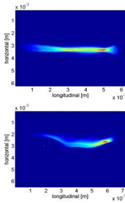
Figure 8: Measured momentum distribution without (top) and with (bottom) strong CSR forces being present.
