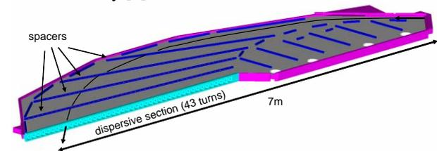
Fig. 2: Layout of 90°-dipole vacuum chamber.
