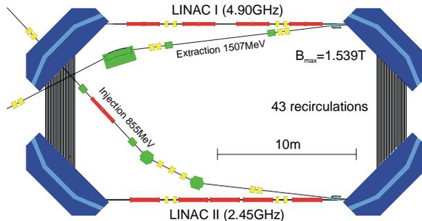
Fig. 1: General layout of the HDSM.
