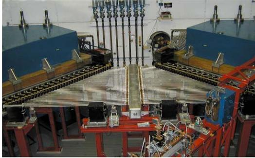
Fig. 3: Return path vacuum system of dipole 3 and 4.
