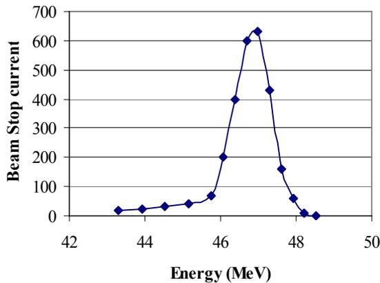
Figure 3: energy dispersion measurement
