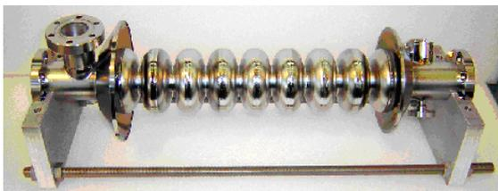
Figure 1: Cavity No.2 before etching.
