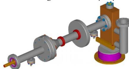
Figure 2: Coupler for 3.9GHz cavity.
