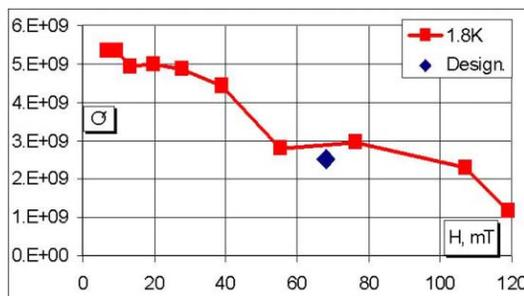
Figure 6: Q and surface magnetic field measured in “0”-mode.
