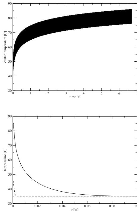
Figure 4: Temperature evolution at the center of the dump window (top) and radial temperature distribution at  $t = 0 \text{ s}$  and  $t = 6.7 \text{ s}$  (bottom).
