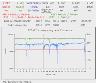
Figure 5: PEP-II's best day showing trickle injection and 844 pb<sup>-1</sup> of integrated luminosity.
