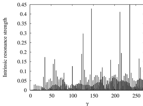
Figure 2: DEPOL calculation of vertical intrinsic resonance strengths for RHIC without snakes. This was for a proton corresponding to a normalized 95% emittance of  $10\pi \times 10^{-6}$  m.
