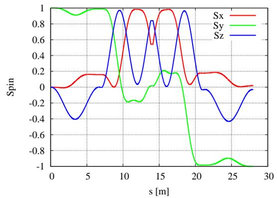
Figure 4: Spin inside 100% helical snake for  $^{241}\text{Pu}^{+94}$  ions at injection ( $\gamma = 10.25$ ) with  $G\gamma = -13.8$ .
