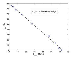
Figure 7: Lorentz Force Detuning vs. field gradient
