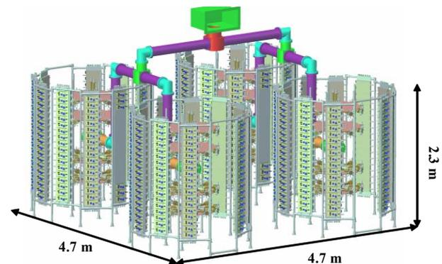
Figure 6 : SR 180 kW amplifier (724 modules of 320 W of which 42 in “stand-by”).
