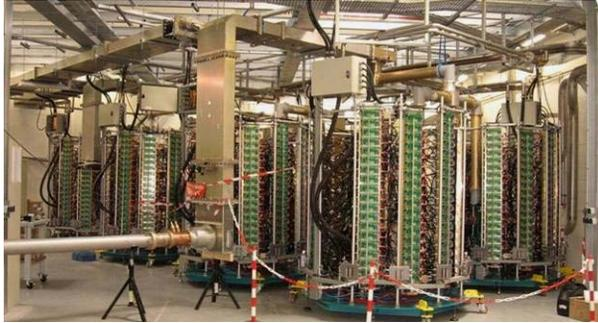
Figure 7: 1<sup>st</sup> SR amplifier under power tests (dummy load).
