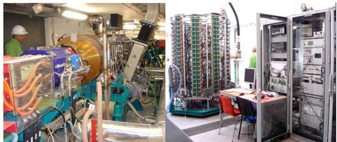
The Fig. 3 above shows a) the cavity in the BO ring and b) the BO RF room with the 35 kW amplifier and the racks containing the control and LLRF systems.
